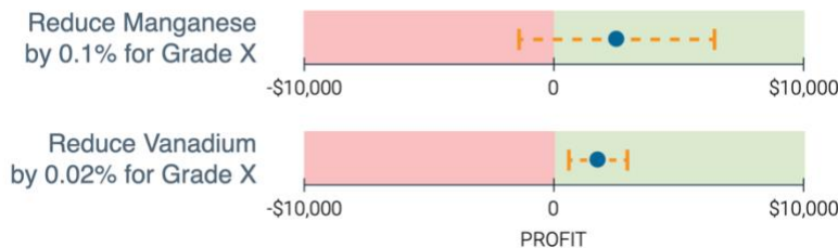
Figure 8: Confidence bands have massive implications on how the ML model's recommendations are used in real world. This figure represents two recommendations with roughly the same mean prediction point (blue dot), and yet with significant difference in confidence band (orange line). In this instance, while the Vanadium recommendation meets the mill's requirements, the manganese suggestion is ignored. The constraints of the requirements can be adjusted on the fly for maximum flexibility and minimum risk.
